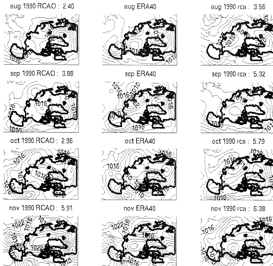
Figure 3. Monthly mean sea level pressure for the coupled model RCAO (left column), ERA40 (center column) and RCA standalone (right column), for months aug, sep, oct, nov. Contour interval: 3 hPa. The coupled model RCAO resembles ERA pressure fields more closely compared to the standalone RCA. The visual impression is supported by RMS differences (in hPa) as given on the right hand side in the titles of the individual figures.
