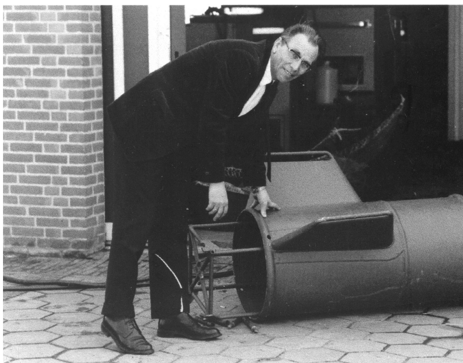
Figure 12-2: J.J. Zijlstra (1926-1989). Director of the Netherlands Institute for Sea Research, showing a plankton torpedo, one of the important tools in biological oceanography
