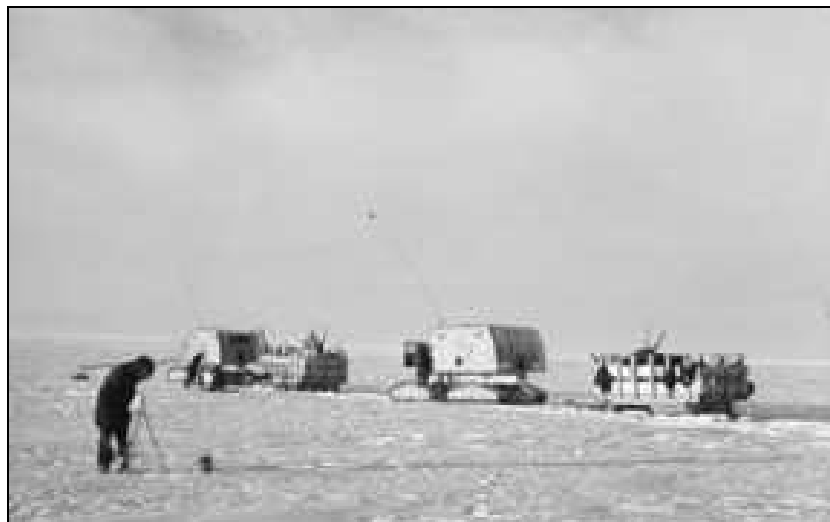
Figure 6-4: Traverse at intermediate station. Behrendt reading magnetometer at left. Walker and Aughenbaugh making snow hardness measurement left background. Thiel on track of Sno-Cat after making a gravity measurement. Crevasse detector visible on lead vehicle (Photograph by John Behrendt).
