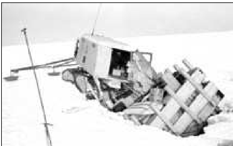
Figure 6-6 (left): Sno-Cat and sled broken into hidden bridged crevasse. Note T-handled probe, ice-axe, and crevasse detector extending forward of Sno-Cat (Photograph by John Behrendt). Figure 6-7 (right): Man trapped in narrow crevasse after breaking through thin snow bridge. He was uninjured and rescued using a wire-rope ladder (Photograph by John Behrendt).
