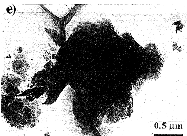
Fig. 5 - TEM images showing: a) at core level 64.58 mbsf, a hairy Fe-rich smectite particle; b) at core level 229.19 mbsf, a hairy Fe-Al smectite particle; c) at core level 252.07 mbsf, a hairy Fe-rich smectite particle; d) at core level 309.74 mbsf, a hairy Fe-Al smectite particle; e) at core level 604.5 mbsf, a hairy smectite developed on a flaky one.
