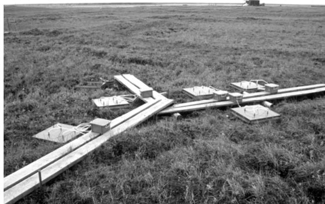
**Figure 7-2:** Measurement field for long term closed chamber flux studies (Samoylov).
