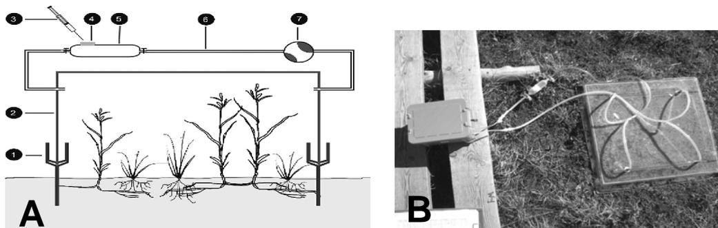
**Figure 7-3:** Scheme of the methane flux measurement set with the closed chamber method (A) and a connected sampling set (B).
