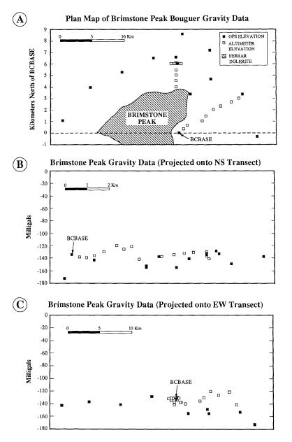
Fig. 2: Map showing Brimstone Peak local gravity survey (A) and gravity profiles of the gravity data projected onto NS and EW lines (B) and (C). Open symbols denote altimeter sites.
