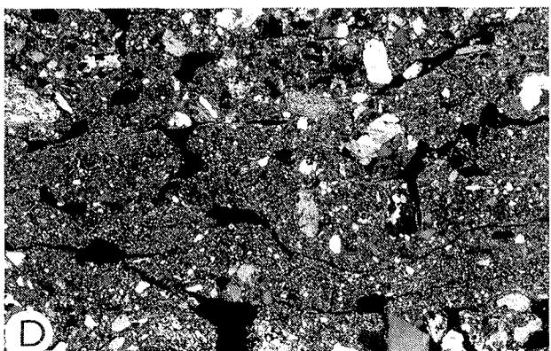
**Fig. 8:** Sample Mi.316. (A) Whole thin section, seen in plane light. (B) Sketch of thin section; rectangles show position of figures (C) and (D); bar indicates 1 cm. (C) Ausschnitt (Bildbreite 11,2 mm) showing mammillated vughs; cross-polarised light; voids in black. (D) Detail (width of view is 11,2 mm) showing flattened nature of pebbles in this sample; cross-polarised light.
