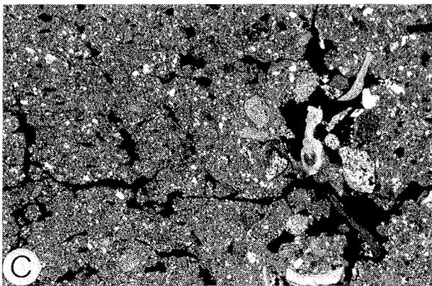
**Fig. 6:** Sample Mi.314. (A) Whole thin section, seen in plane light. (B) Sketch of thin section, dotted line represents calcitan; rectangle shows position of figure (C); bar indicates 1 cm. (C) Detail (width of view is 18 mm) showing suggested welded pattern of pebbles, notice detached calcitans; cross-polarised light; voids in black.
