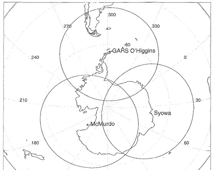
**Fig. 1:** Ground station coverage of X-band-receiving stations in Antarctica for ERS-1/2 (visibility circles).
