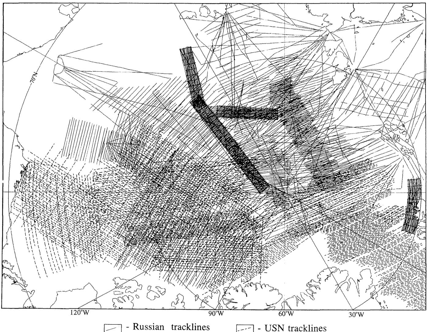
Fig.1: Russian and US Navy aeromagnetic tracklines in the central Arctic seas.
