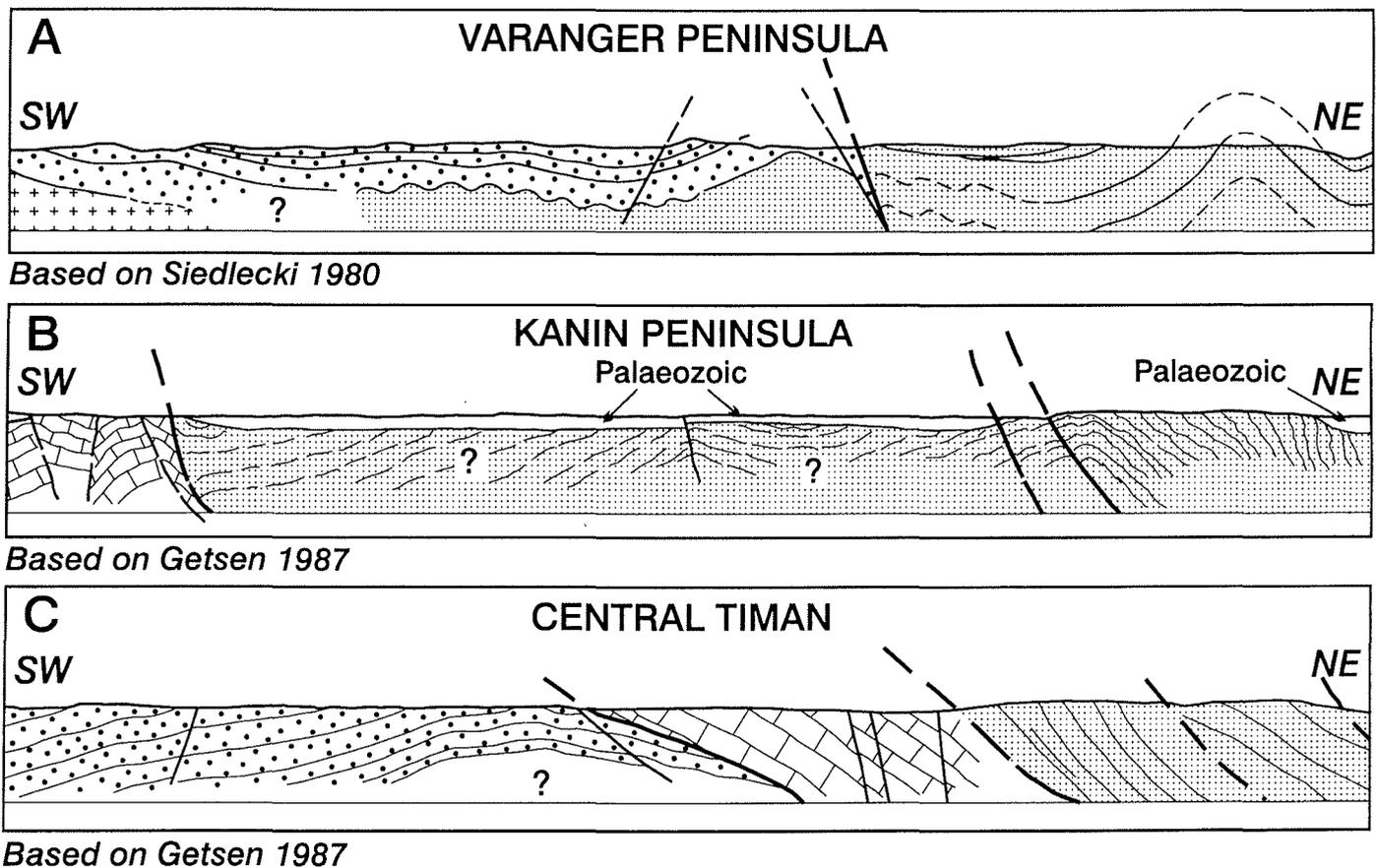
Fig. 3: Summary cross sections showing the main features of the structure in the Timan-Varanger Belt (not to scale).
