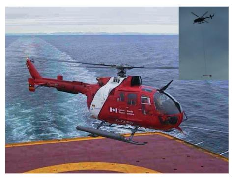
**Fig. 6:** Helicopter taking off for aeromagnetic survey flight (inset with bird) from the helideck of the CCG "Louis S. St. Laurent".
