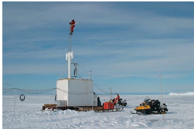
Fig. 8: The hydro-acoustic observatory (PALAOA) is closely located to the ice-shelf edge. The underwater sound is continuously recorded with four hydrophones installed in the water below the 100 m thick ice-shelf sheet.
