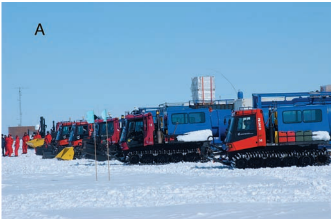
Fig. 12: The tracked vehicle fleet at NM-II consists of eleven Kässbohrer “Pisten Bully” (PB 260 and PB 300).
