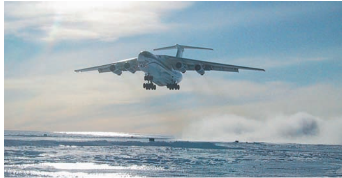
Fig. 15: Iljushin (IL-76TD) take-off from Novo-Runway (70°51'S, 011°36'E), which is located on the inland ice at an elevation of 550 m ASL about 15 km southward of the Russian station Novolazarevskaya in the Schirmacher Oasis. The landing strip is prepared by compacted snow and certified for landing of heavy wheeled cargo aircraft such as IL-76TD or Hercules C-130. The size of the runway is 2980 m by 60 m. Since season 2002/2003 Novo-Airbase is operational every year from the beginning of November until mid-February.
