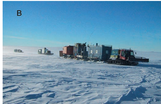
Fig. 12: The tracked vehicle fleet at NM-II consists of eleven Kässbohrer “Pisten Bully” (PB 260 and PB 300).
