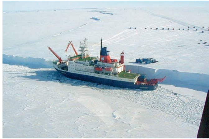
Fig. 10: Supply of Neumayer Station II (NM-II) by ship, unloading of RV "Polarstern" dynamically moored to the edge of the Ekström Ice Shelf near Atka Bay (for location see Fig. 22).
