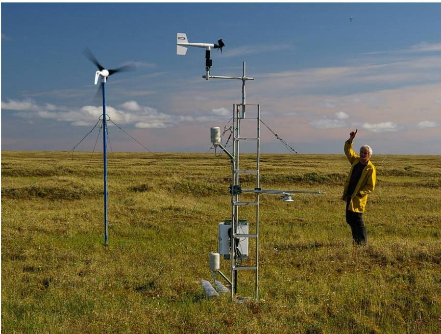
**Figure 3.2-2:** Metreological station for the observation of standard climate parameters like air temperature, humidity, soil surface temperature, wind speed and direction, precipitation and snow height.
