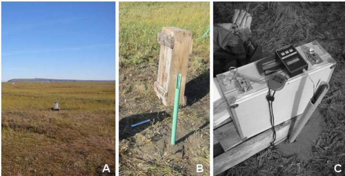
**Figure 3.5-1:** Methane gradient analysis in the perennially frozen ground: A: study site on Samoylov Island, Lena Delta; B: tube of the installed GASSYS system for gas sampling and C: pressure measurements.
