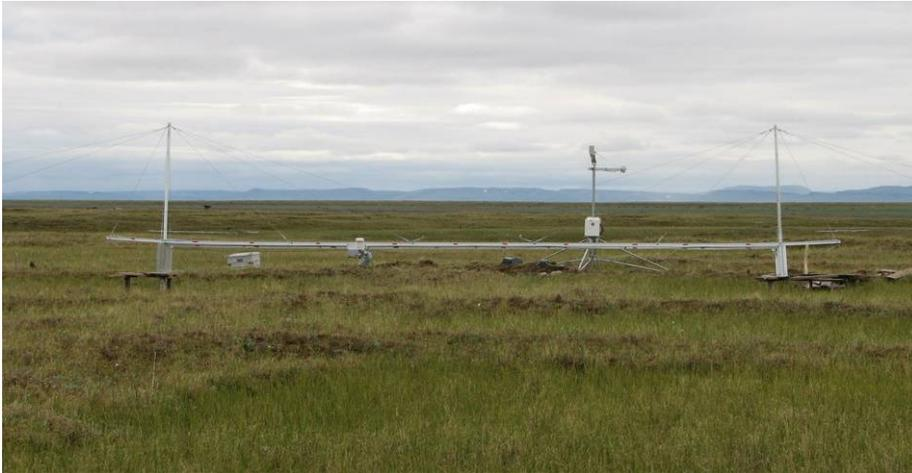
**Figure 3.2-1:** Radiation Scanner System for measuring differences in the outgoing short and long wave radiation. The scanner track is 10 meters long and crosses two adjacent polygons. Soil temperature and soil moisture probes underneath the scanner track observe differences in ground heat fluxes.
