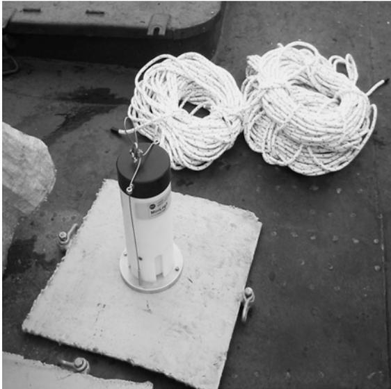
**Figure 3.9-1:** A data logger, attached to a steel plate fitted with attachment rings for the ropes in the background, on board the “Puteyski 405” in preparation for deployment.
