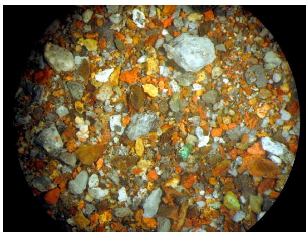
Fig. 1.75: A microscopic view of a sulfidic hydrothermal sand rich in heavy metals
