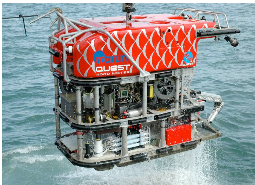
Fig. 1.48: ROV "QUEST" with KIPS mounted on the starboard side of the tool sled
