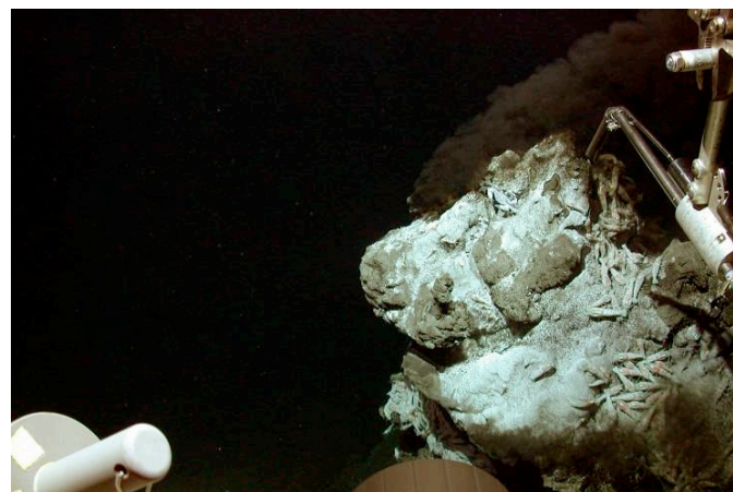
Fig. 1.50: Measured in-situ temperatures during fluid sampling with KIPS at Mephisto Ven , Red Lion, orifice on top of the chimney. Maximum temperature measured was 346.3 °C, at a water depth of 3098 m. Samples 7 ROV-1 to -3 were taken from 7:50 – 18:08 UTC.
