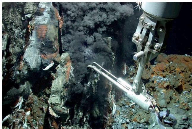
Fig. 1.49: Measured in-situ temperatures during fluid sampling with KIPS at Marker #2 Vent , Turtle Pits, in an orifice approx. 1 m above ground. Maximum temperature measured was 395.1 °C (note unstable temperature readings, compare to Fig.1.53), at a water depth of 2986 m. Samples 3 ROV-10 and -11 were taken from 21:30 – 21:45 UTC.
