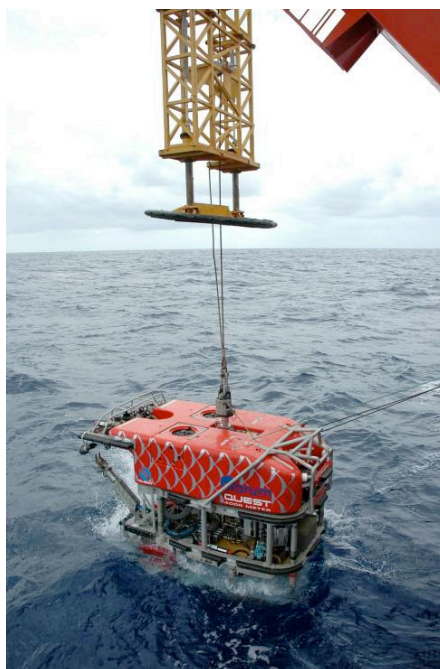
Fig. 1.8: MARUM ROV "QUEST4000m" deployed from the A-frame mounted launch and recovery system (LARS) behind the stern of R/V METEOR.
