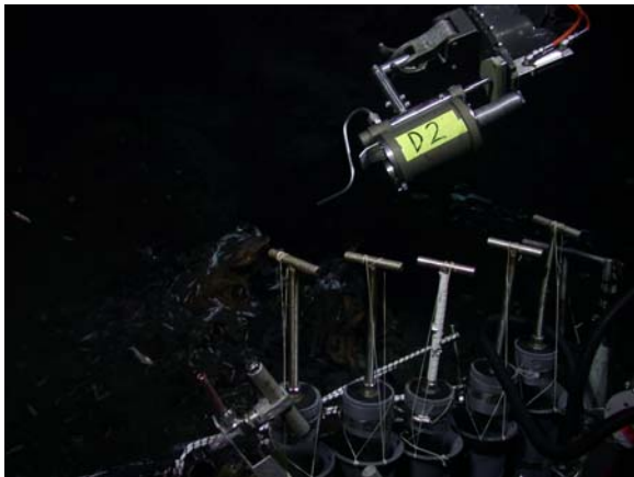
Figure 3-22: “Major” water sampler operated by the ROV manipulator arm.
