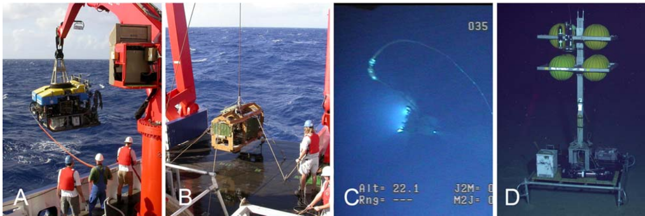
Figure 3-6. The ROV Jason II. A: Launching of the vehicle Jason II; B: launching of Medea; C: View from Medea on Jason II during operation on the seafloor; D: Free-fall elevator.
