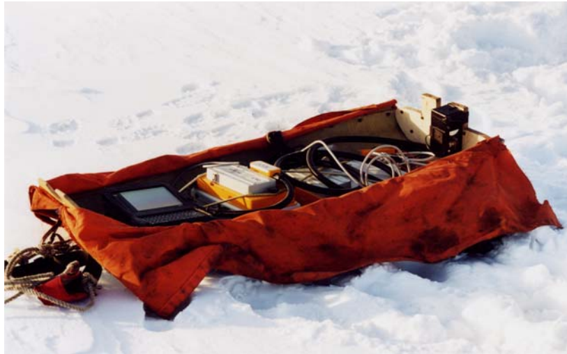
Figure SEAICE.17: The RAMAC GPR mounted into a little Pulka.
