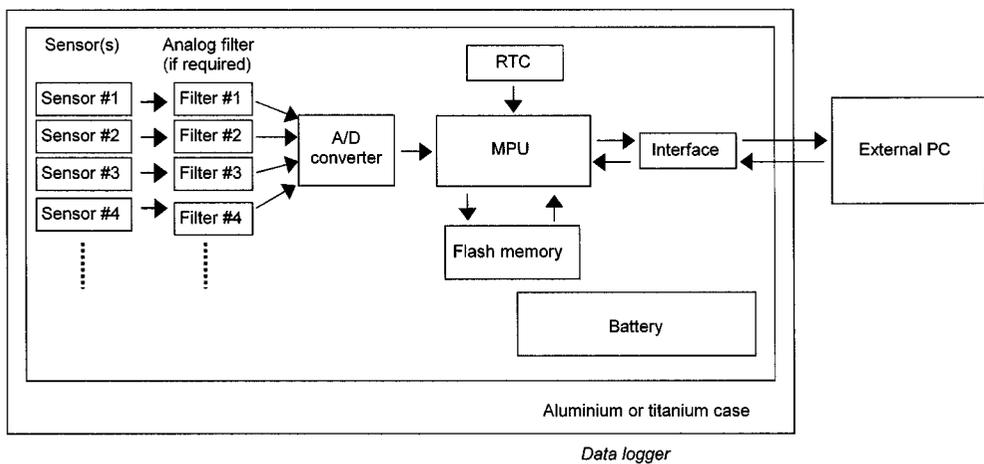
Fig. 1. Schematic diagram of Little Leonardo data logger.
