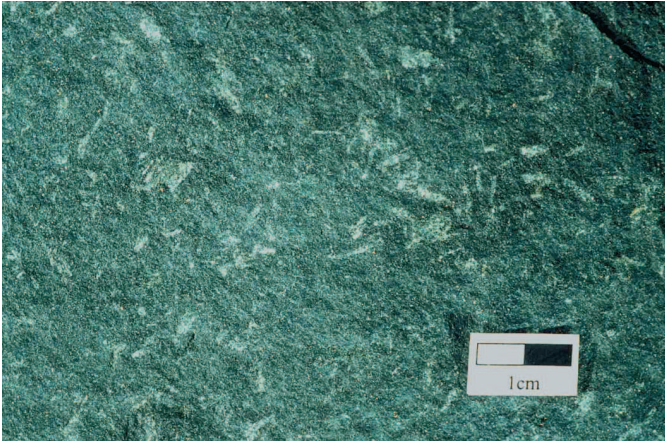
Fig. 4: Sample KF89 (Christophersennabben, Sivorgfjella) showing a subophitic texture. The feldspar crystals are completely replaced by albite, clinozoisite, quartz, and white mica.
