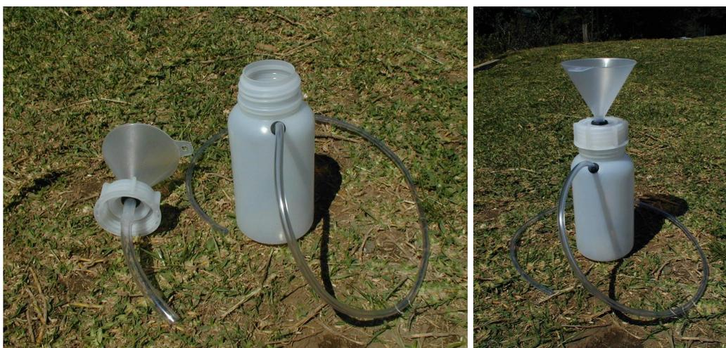
**Figure 2.13:** Rainwater sampler for isotopic analysis. The hose connected to the funnel goes down to the bottom of the bottle so that the first precipitation prevents further contact of the sampled water with the atmosphere.
