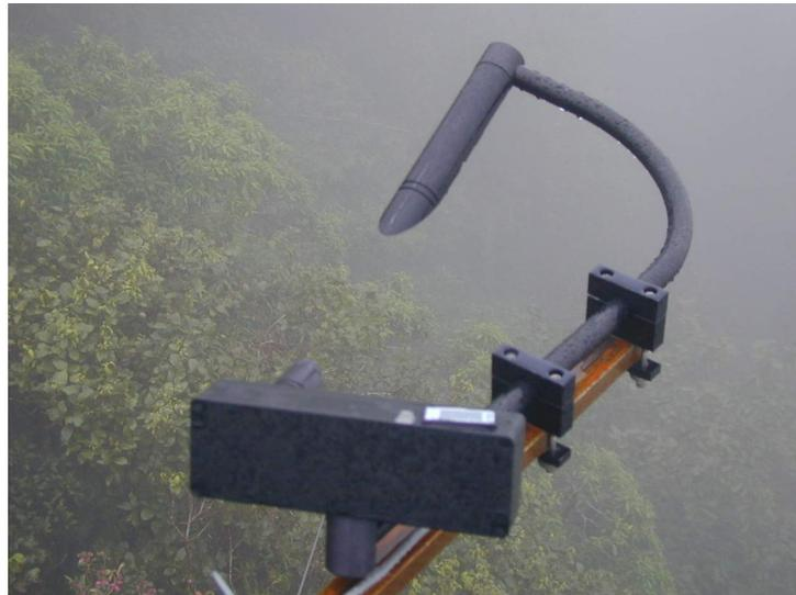
**Figure 2.4:** *Present weather detector (PWD11 manufactured by Vaisala, FI).*
