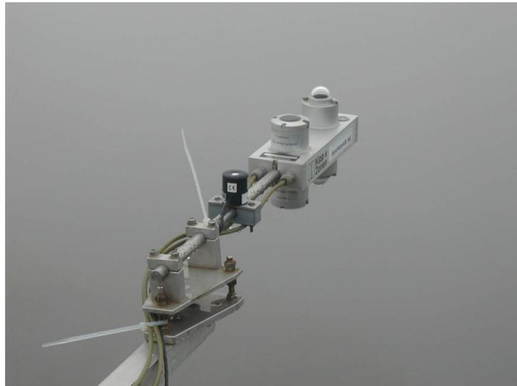
**Figure 2.3:** Kipp & Zonen CNR1 net radiometer and PAR sensor (Skye SKP215 PAR quantum sensor).
