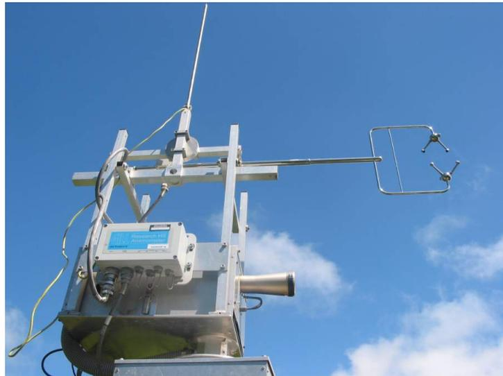
**Figure 2.9:** *The eddy covariance measurement set-up: Ultrasonic anemometer (horizontally) and an active high-speed FM-100 cloud particle spectrometer (bottom part, funnel visible at the right side).*
