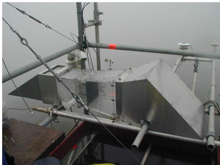
**Figure 2.12:** *Caltech Active Strand Cloudwater Collector.*
