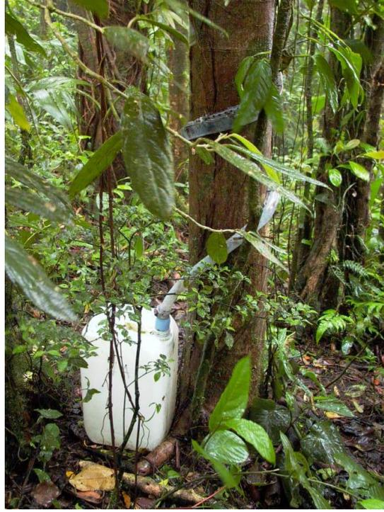
**Figure 2.11:** *Stemflow measuring installation.*
