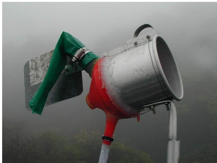
**Figure 2.6:** *Self constructed vertical-orifice-gauge for wind-driven rain at the top platform of the meteorological tower (UFO).*
