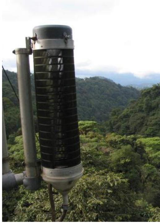
**Figure 2.7:** Modified Juvik horizontal precipitation gauge mounted at the meteorological tower (24 m height)(photo by Arnoud Frumau).
