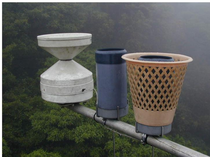
**Figure 2.5:** *One automatic (white) and two totalizing rain gauges at the top platform of the meteorological tower.*
