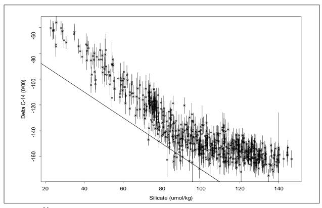
**Figure 3:**  $\Delta^{14}$ C as a function of silicate for S4P AMS samples. The straight line shows the relationship proposed by Broecker, *et al.*, 1995 ( $\Delta^{14}$ C = -70 - Si with radiocarbon in % and silicate in  $\mu$ mol/kg).
