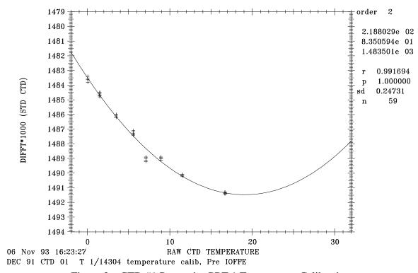
Figure 2a: CTD #1 Pre-cruise PRT-1 Temperature Calibration
