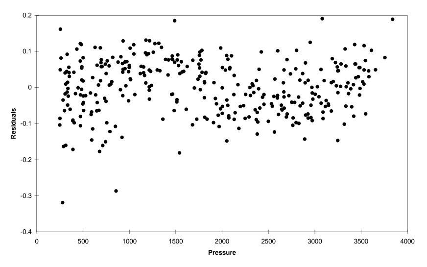
Figure 4. Residuals remaining after the calibration has been applied to the down cast CTD oxygen data.
