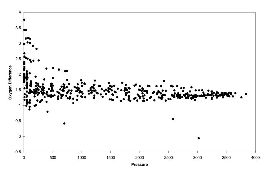
Figure 1. Water sample oxygen data minus the down cast CTD data,  $d_{ij}$ , plotted against pressure.
