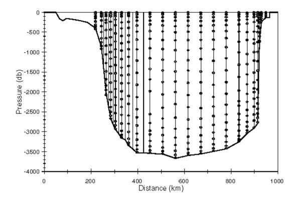
**Figure 7.** 1994 Bottle and CTD Positions. CTD profiles without bottles are indicated by vertical lines only. Bottle trips are indicated by solid dots.
