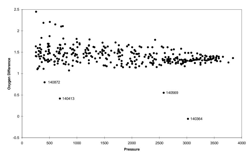
Figure 2. Oxygen differences,  $d_{ij}$ , plotted against pressure for data points having a pressure below 250 dbars.
