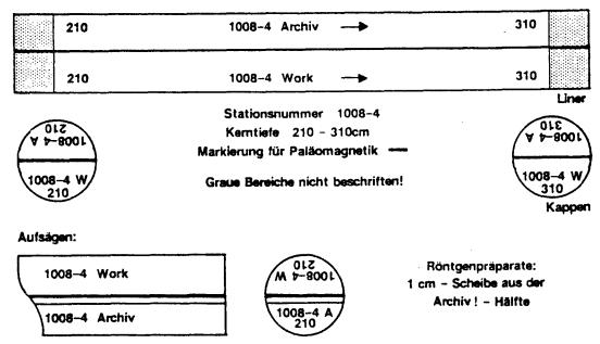
Fig. 35: Labeling for the plastic liners of the gravity core
