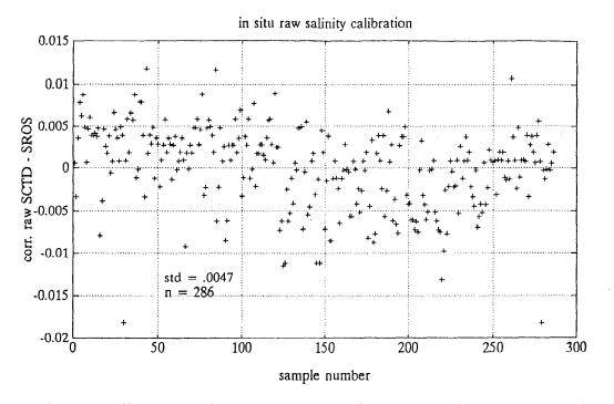
Fig. 8: Salinity differences after calibrating the CTD salinity (not conductivity).
