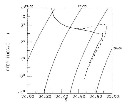
Fig. 13: Potential temperature (°C) plotted against salinity (psu) for deep water colder than 4°C. Station 42 in the Vema Channel is shown for comparison (dashed).
