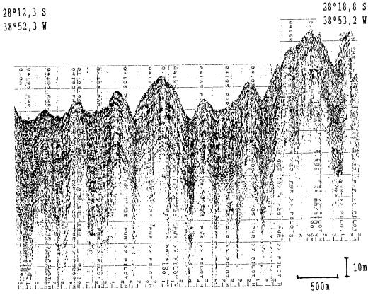
Fig. 33: Sediment waves north of the Vema Channel. Different wave lengths and amplitudes show sediment transport by bottom water current.
