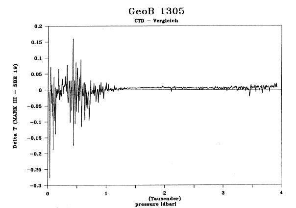
Fig. 37: Comparison of the temperature profiles of the Mark III and SBE 19-2 at station GeoB 1305 (station 85)
