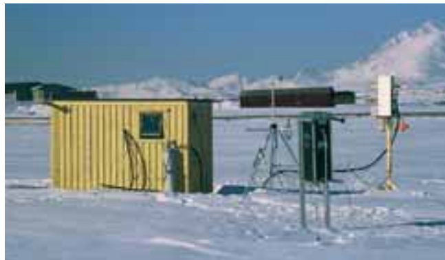
Measuring devices from the University of Grenoble document mercury pollution of snow and atmosphere during the Arctic spring. (Photo: Christophe Ferrari)
