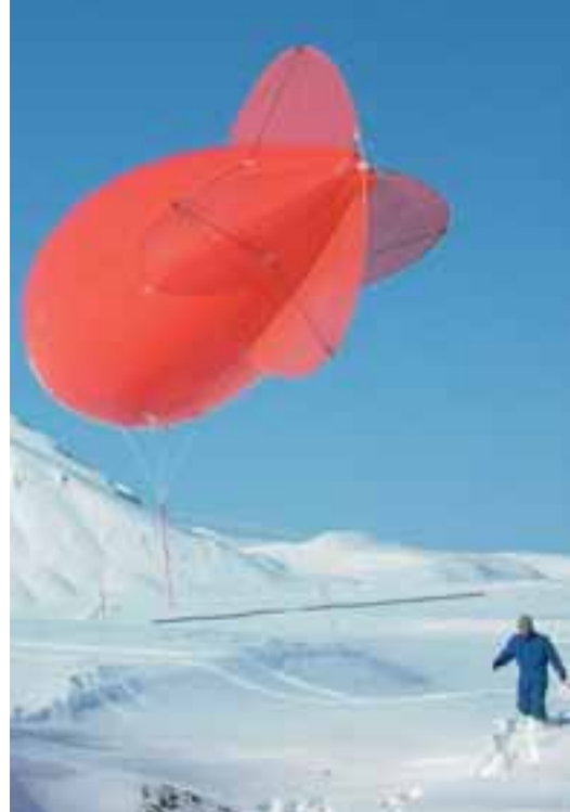
Rising balloons equipped with data loggers record vertical stratification in the atmosphere, up to three kilometres altitude. They are released from the balloon house of the Atmospheric Observatory and provide weather data such as air pressure, temperature, humidity and wind speed. (Photo: Anne Hormes)
