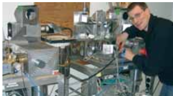
The station engineer looks after technical maintenance of the microwave radiometer used in the identification of atmospheric gases such as water vapour and ozone. (Photo: Bettina Saier)
