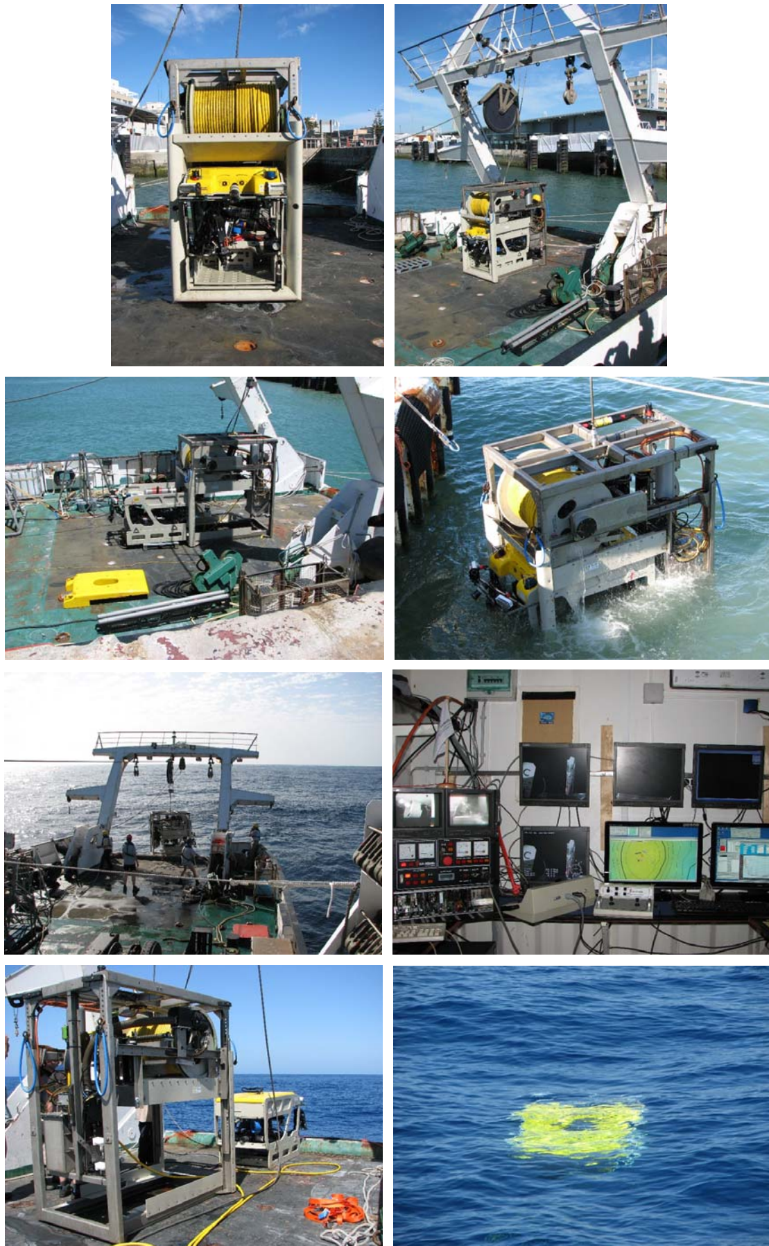
Figure 4: Pictures demonstrating the ROV deployment and operational environment.
