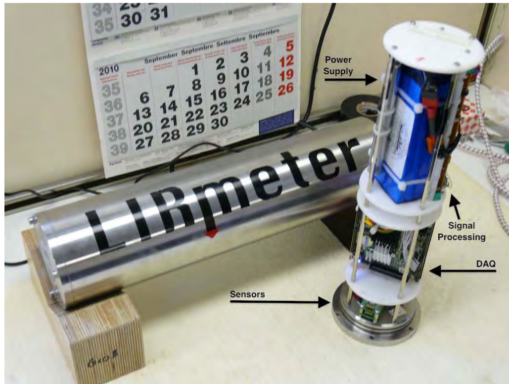
Figure 13: Left: LIR-Meter in pressure casing; right: electronics
