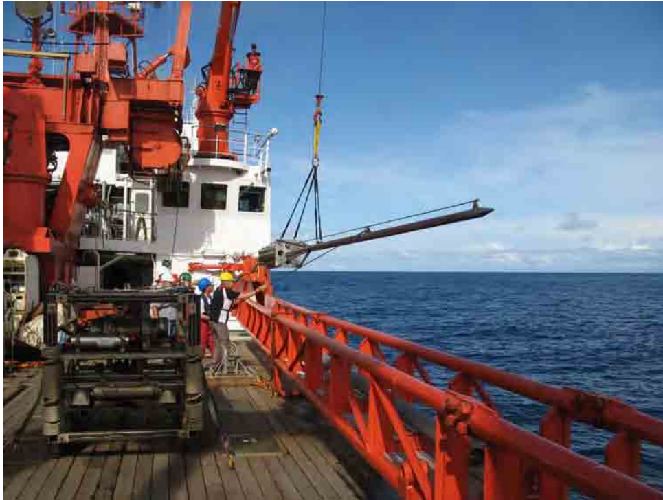
Figure 10: The 6 m Bremen Heat Flow Probe on deck during cruise SO207.
