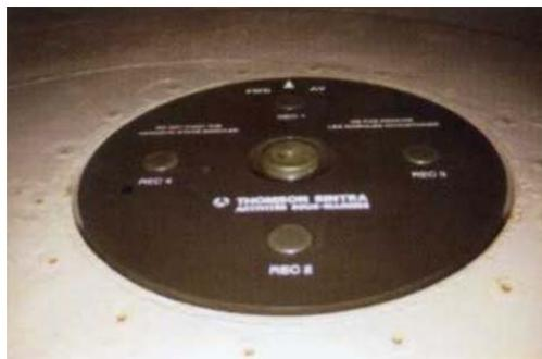
**Figure 3.11:** POSIDONIA acoustic array – flush version,  $\varnothing$  80 cm (after Bellier, 2002).
