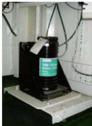
**Figure 3.9:** Heave compensator.
