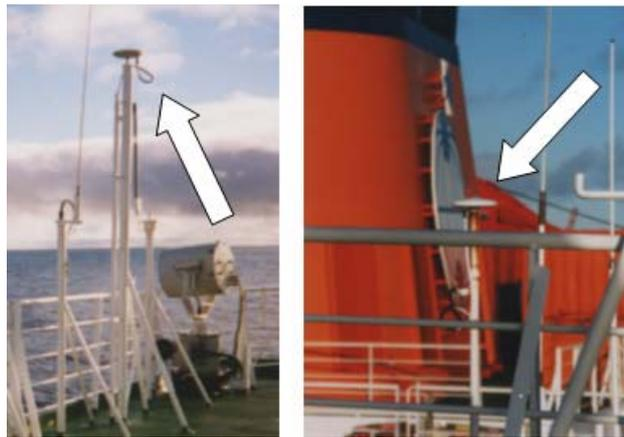
**Figure 3.2:** One of the TRIMBLE antennas (left) and the LEICA antenna (right) on board POLARSTERN (2002).
