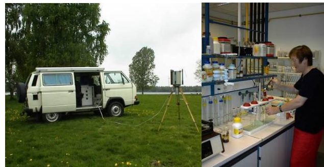
Figure 5-1: Left: Field gamma-spectroscopy during the routine monitoring program. Right: Chemical extraction of radionuclides for alpha spectroscopy.
