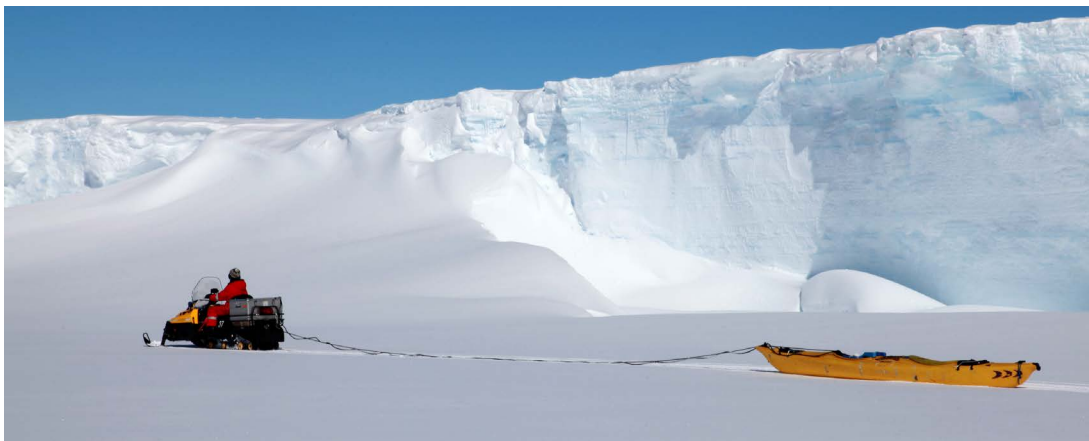
Figure 8: EM31 pulled behind snowmobile
