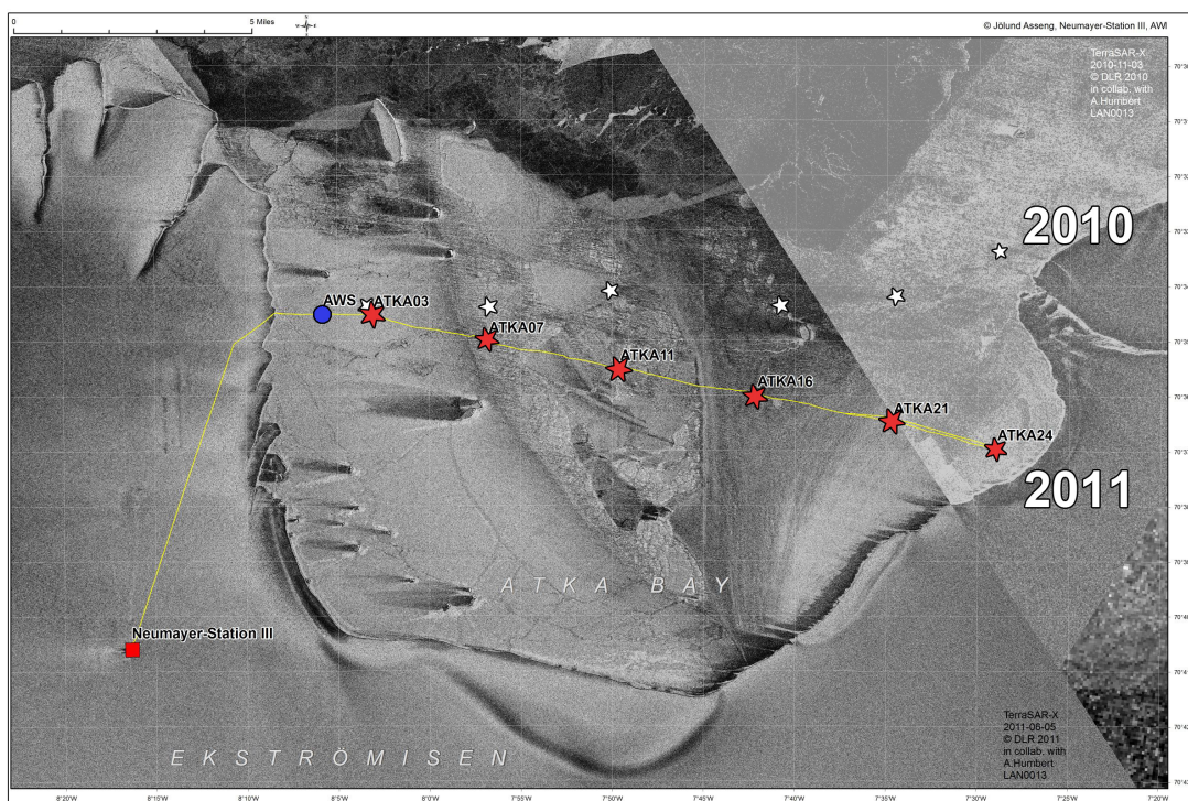
Figure 2: TerraSAR-X image of Atka Bay with stations of AFIN measurements in 2010 (white stars), 2011 (red stars) and the site of the automatic weather station and thermistor chain (blue dot). Station names (e.g. ATKA03) refer to the distance to the western ice-shelf edge.
