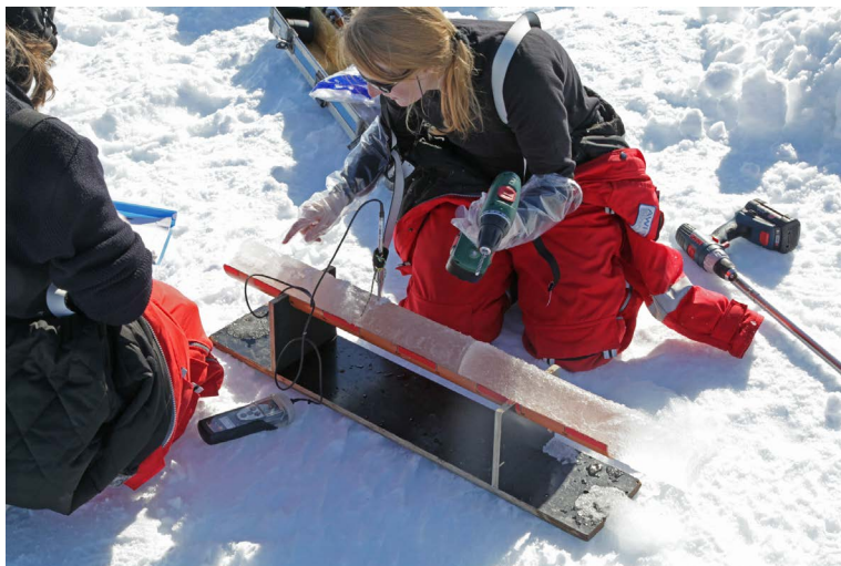
Figure 26: Measuring the temperature of a sea-ice core
