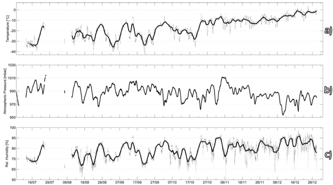
Figure 16: Atmospheric conditions at AWS site (Figure 2), measured by Automatic Weather Station in 2011 (gray line) and daily running mean (black line). a) 2m air temperature; b) air pressure; c) relative humidity.
