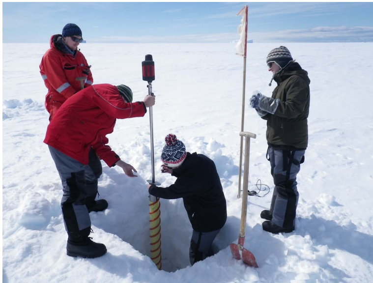
Figure 25: Retrieval of a sea-ice core with a Kovacs Mark II coring system
