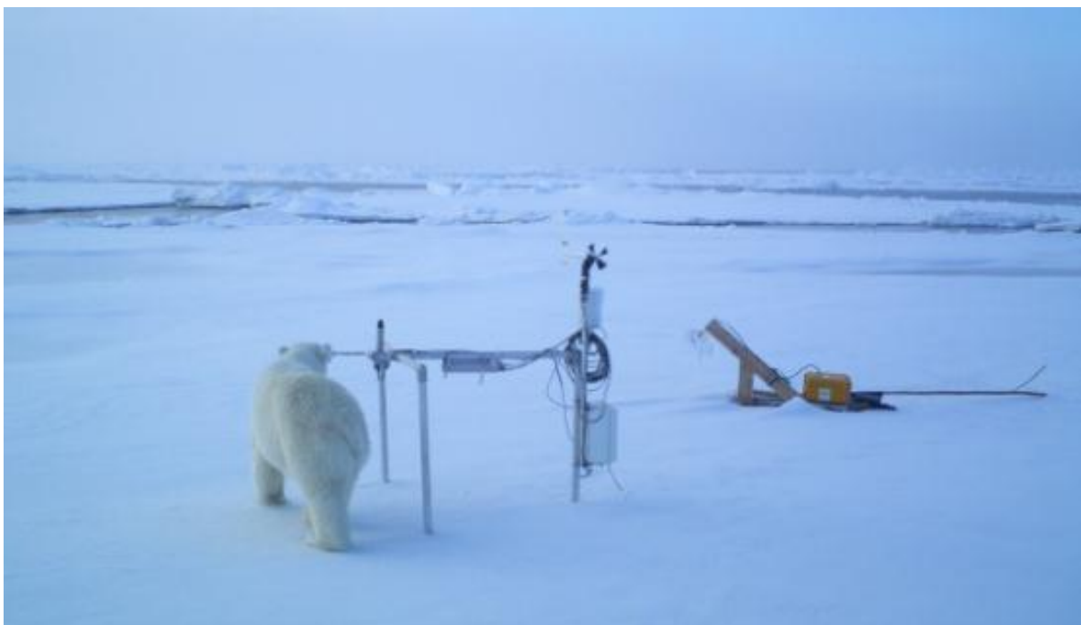
Figure 17: On 9 th September 11:30 (UTC), the station got visited by an interested polar bear. He stepped over the flag visible in the right and ripped the cable of the temperature and humidity sensor. The picture taken by the automated camera shows well the changed surface conditions, though the pond is still visible to the left as a depression in the snow surface. The camera stopped working ten days before retrieval.
