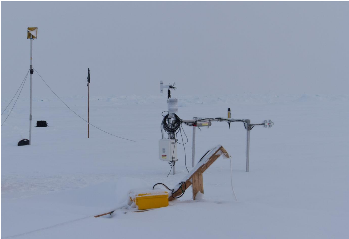
Figure 20: Images of the long-term installations before retrieval. SAMS-IMB (top left), the pressure ridge marked with flags and SVP (top right) and the weather and radiation station after retrieval of the datalogger (bottom).
