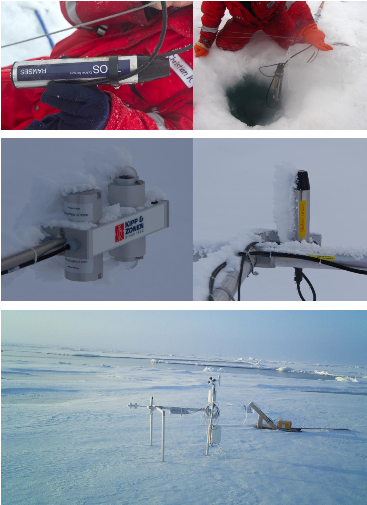
Figure 23: Algae cover growing on the upper side of the under-pond sensor is visible after retrieval (top left). Retrieval of under-ice sensor (top right). Albedometer before retrieval covered in rime (middle left). Surface RAMSES sensor before retrieval (middle right). Last picture taken by the automatic camera on 18 th September (9:30 UTC) 10 days before pickup.
