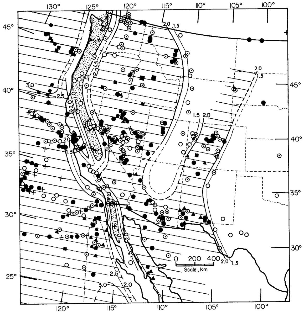
FIGURE 2. Heat flow map of western United States (Roy *et al.*, 1972). Pluses represent heat flow values in the range of 0 to 0.99; open circles, 1.0 to 1.49; dotted circles, 1.5 to 1.99; solid circles, 2.0 to 2.49; solid triangles, 2.5 to 2.99; solid rectangles, >3.0.
