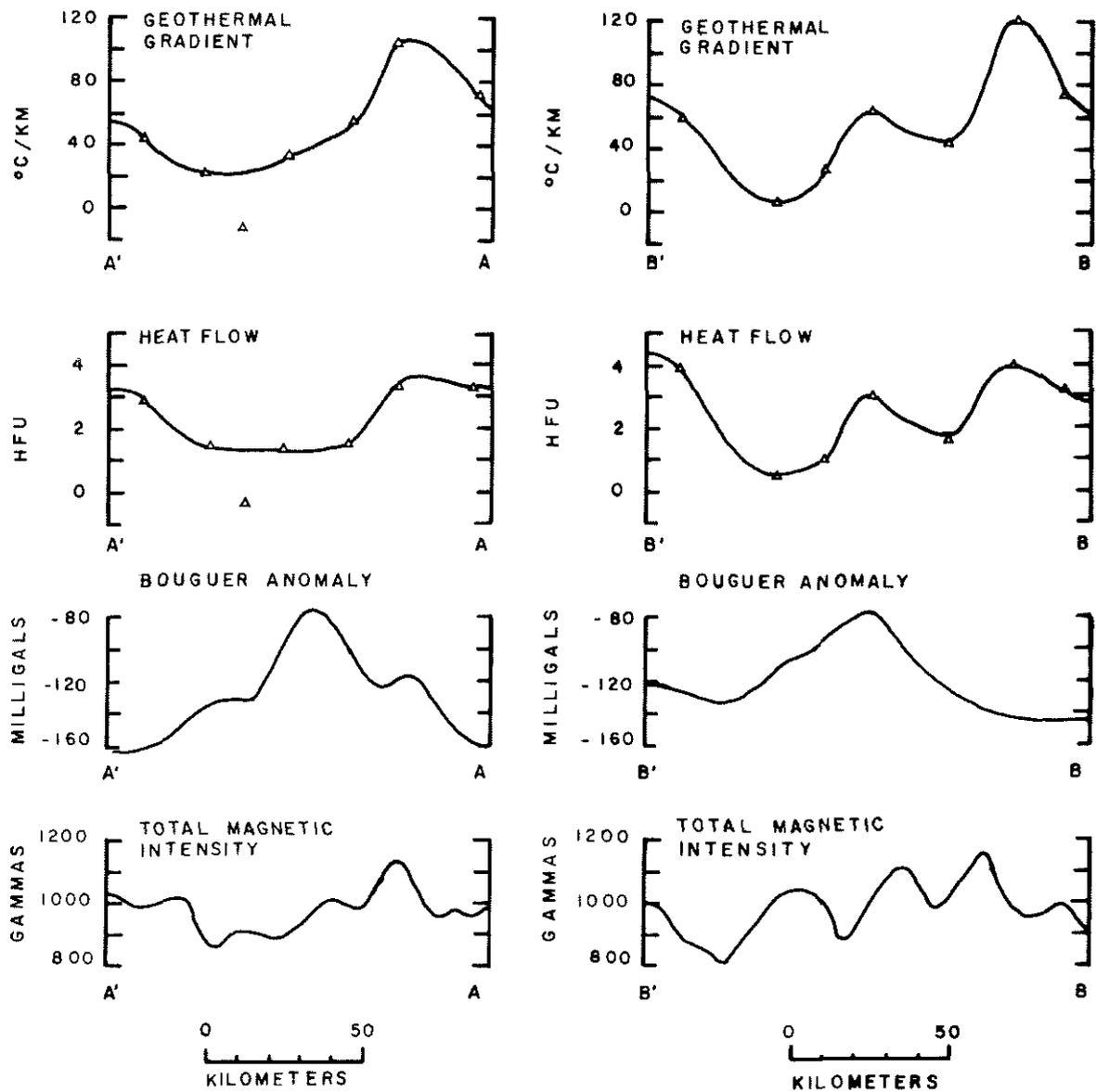
FIGURE 11. Geothermal gradient, heat flow, Bouguer gravity and residual magnetic north-south profiles A'A and B'B) across the Snake River Plain. The gravity and magnetic profiles are from Mabey (1976).
