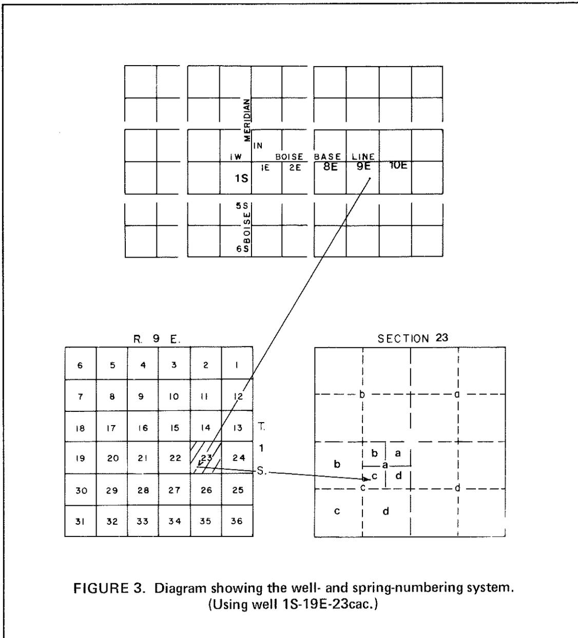
FIGURE 3. Diagram showing the well- and spring-numbering system. (Using well 1S-19E-23cac.)
