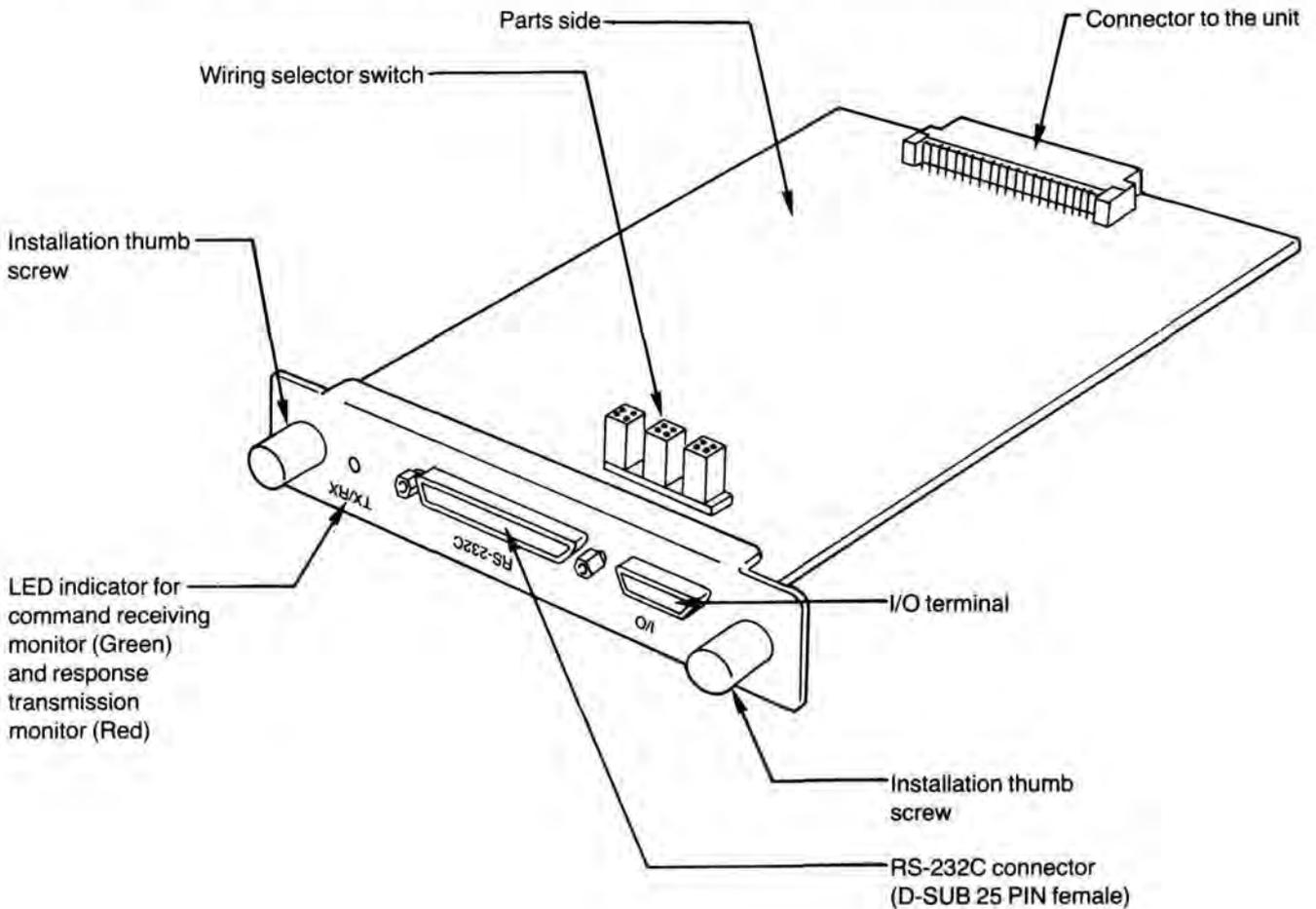
2) Wiring selector switch set up
