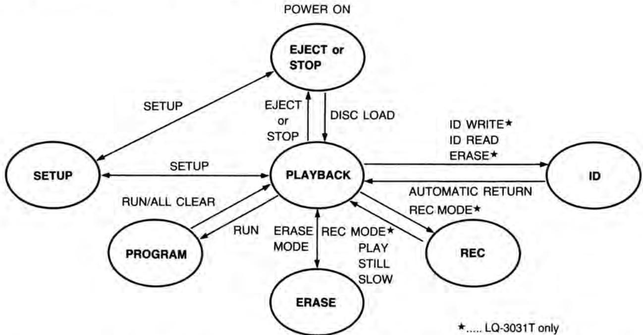
■ As shown in above diagram, SETUP button is effective only when in the Off-line Mode, and Eject, Stop and Playback Modes. When SETUP button is pressed, it toggles SETUP mode set up/clear.
