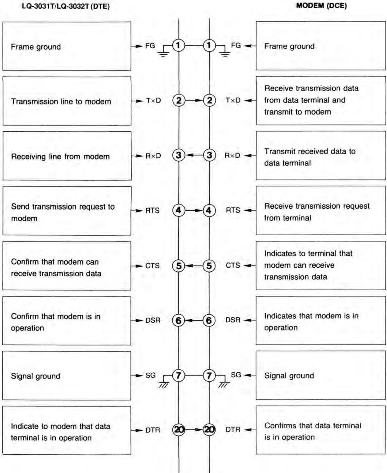
**7. CONNECTION WITH DATA TERMINAL EQUIPMENT (DTE)**
