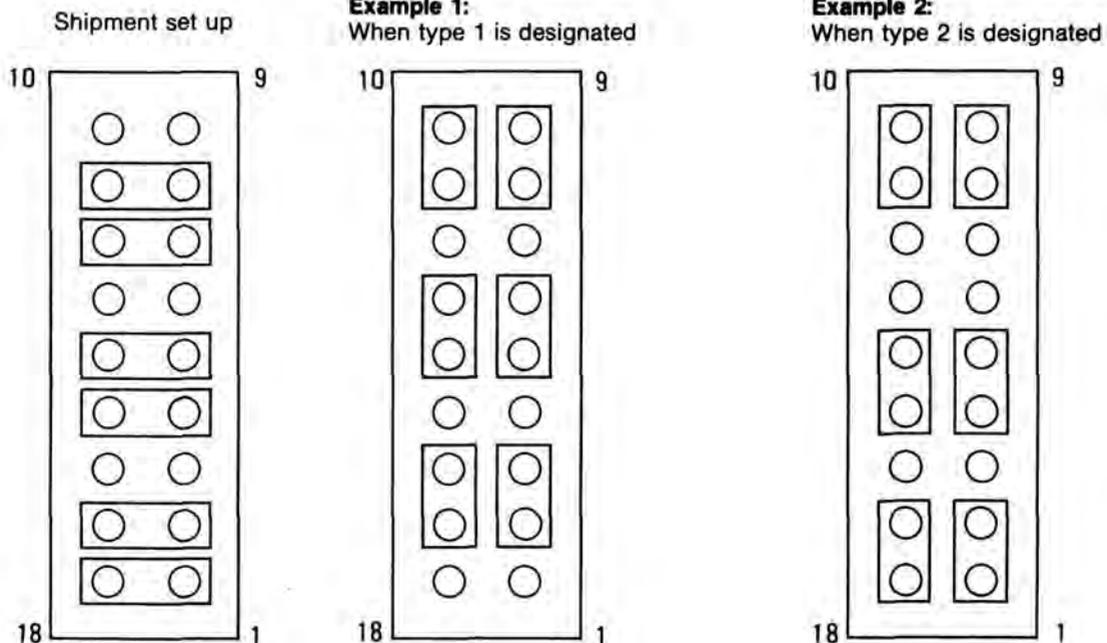
\* Wiring selector switch is straight wired at time of shipment. When DTE terminal by straight RS-232C cable, wiring selection should be done as examples indicate.
