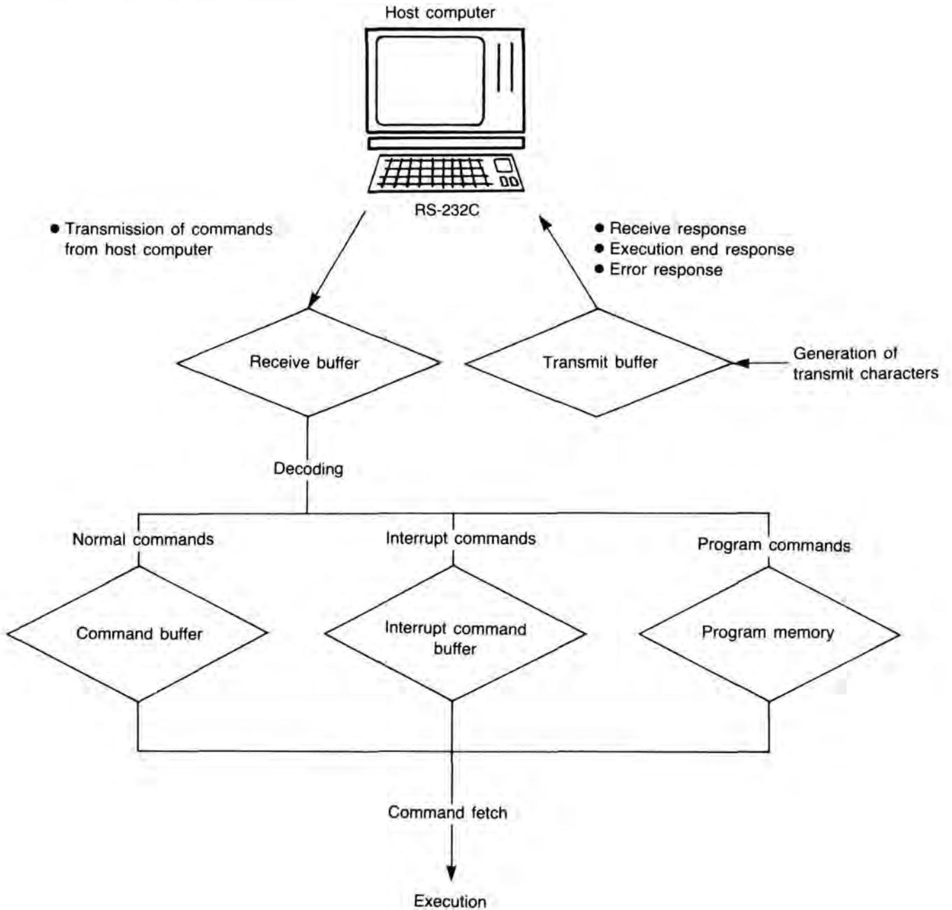
**Note:** When receiving the program run command, the unit fetches commands from the program memory for execution, and in response to the other commands, it fetches commands from the command or interrupt buffer for execution. The commands in the interrupt command buffer are executed prior to those in the command buffer.
