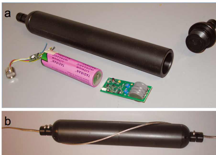
Fig. 1. (a) The probe housing and its internal components (from left to right: pressure transducer, lithium battery, transmitter). (b) A probe attached to the 3 mm Kevlar rope using rope clamps attached at both ends of the housing.
