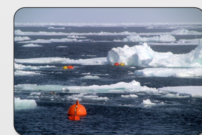
Left: bright and colorful floatation enhances detectability of moored recorders upon retrieval in ice covered areas; Right: flags mark on-ice recorder positions, light-colored recorder casing limits melt-in
