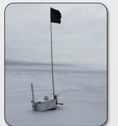
Left: bright and colorful floatation enhances detectability of moored recorders upon retrieval in ice covered areas; Right: flags mark on-ice recorder positions, light-colored recorder casing limits melt-in
