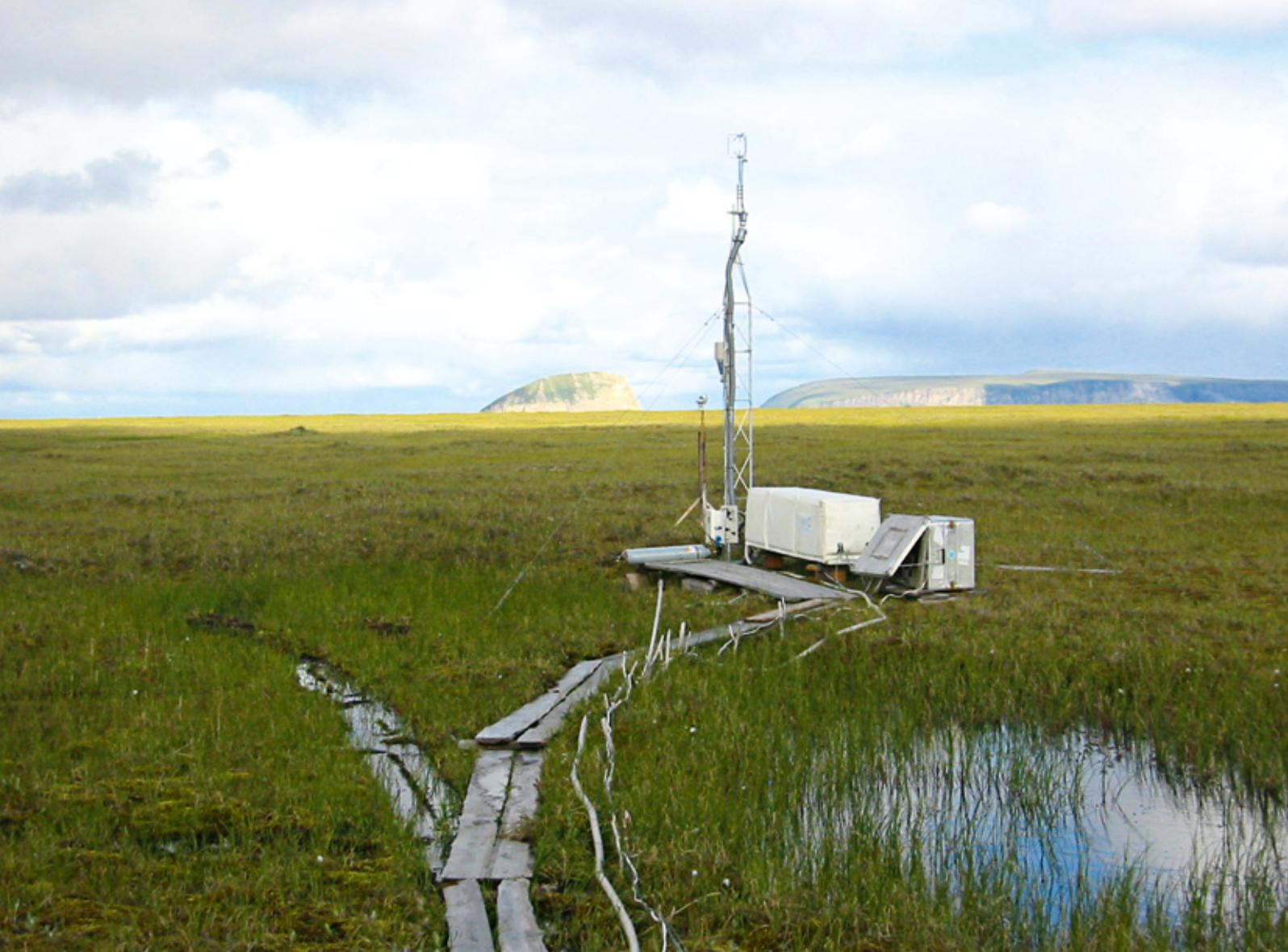
*Fig. 3.3: Micrometeorological system for temporally and spatially highly resolved measurements of greenhouse gas fluxes between tundra and atmosphere in the Lena River Delta, Siberia. (Photo: Torsten Sachs)*
