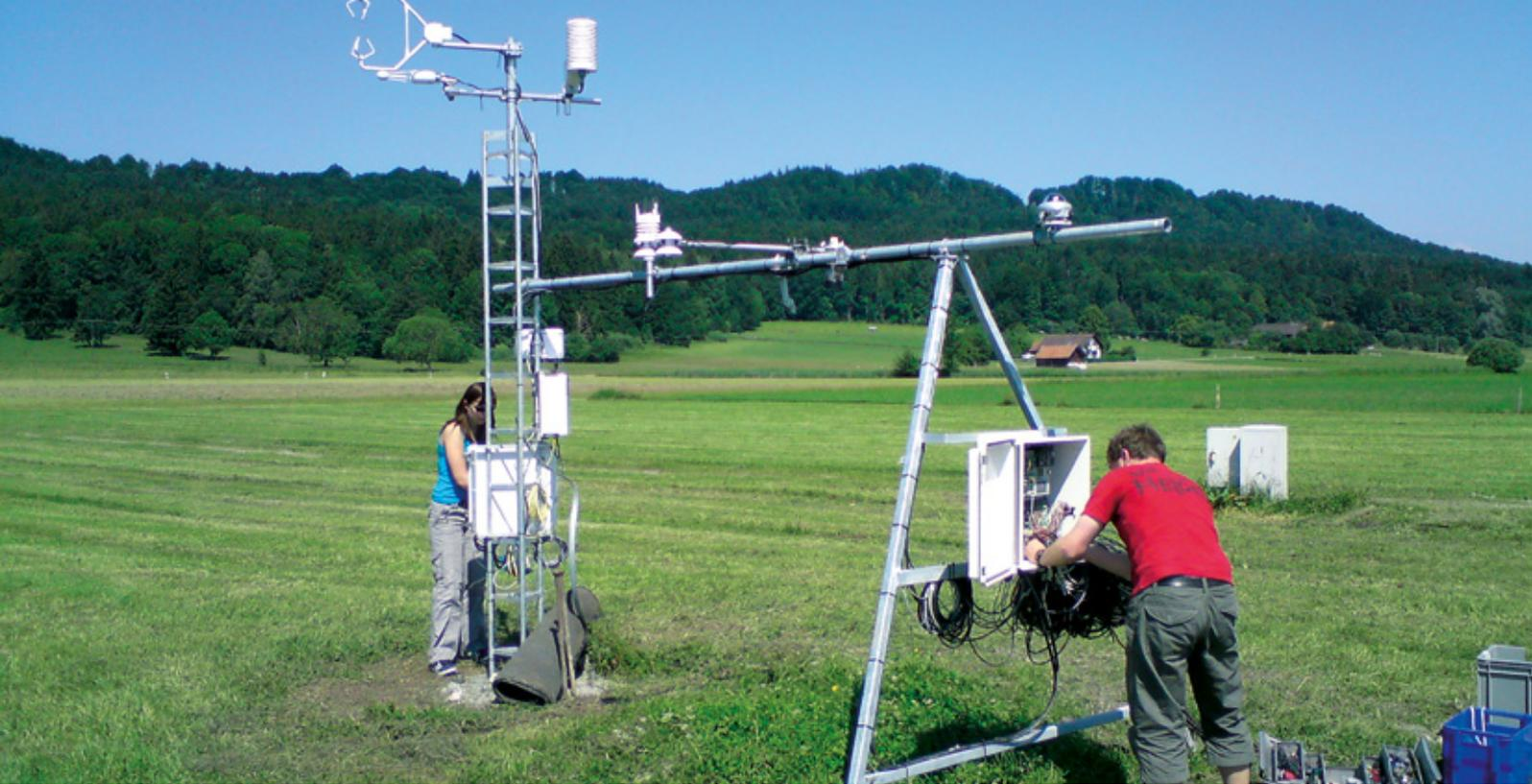
Fig. 4.2: C. Jahn and K. Heidfeld at the final installation of the Fendt eddy-covariance measurement station in the TERENO pre-alpine observatory. (Photo: Matthias Mauder)
