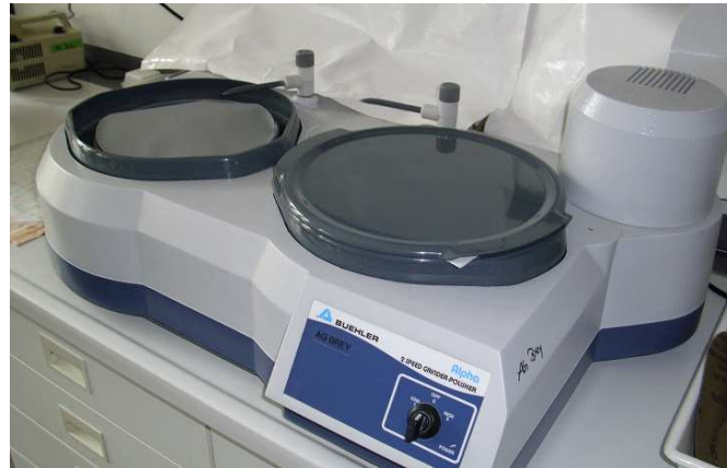
Abb. 8: Schleifmaschine Buehler Alpha wheels, 2 speed grinder polisher.
