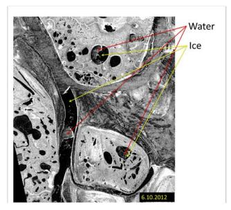
Figure 3 TerraSAR-X image subset. Clear backscatter differences are visible on the water bodies. Dark areas represent areas covered by thin ice, lighter areas display wind effected water surfaces.
