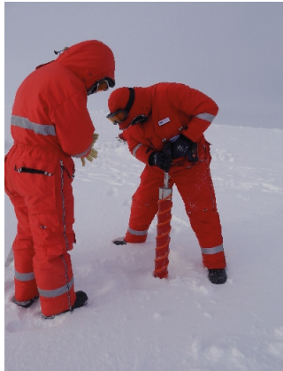
Fig. 6.4.1: Drilling of ice cores (photo Jörg Göttlicher)
