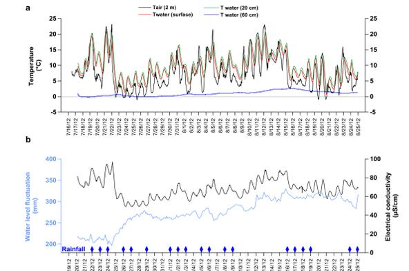
**Figure 5** Monitoring data obtained from the site POK-01 from July 16 to August 25, 2012. (a) Air and water temperatures; (b) Electrical conductivity, water level, and rainfall.
