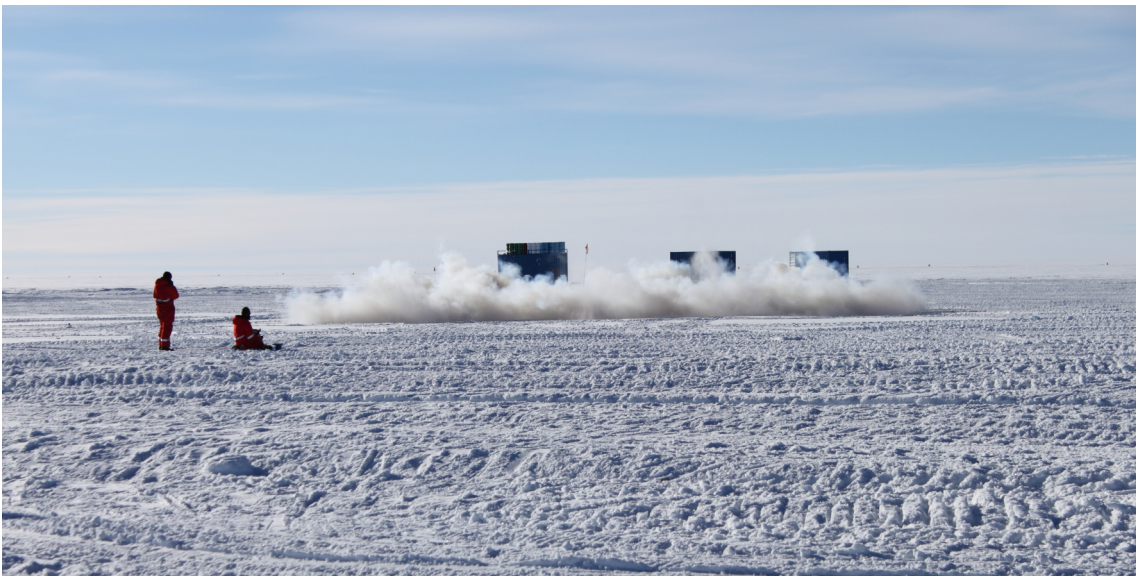
Figure 1.2.: Explosive shot using detonation cord at the surface close to Kohlen station, Dronning Maud Land, Antarctica.
