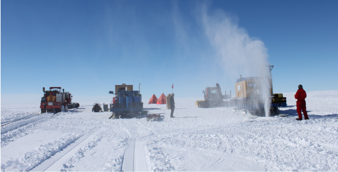
Figure 1.1.: Field camp at Halvfarryggen, Dronning Maud Land, Antarctica with vibrator truck (red vehicle on the left side) and ongoing drilling with air-pressure drill (right side).
