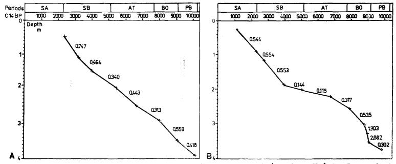
Fig. 4. Graph showing the accumulation rate of peat-bog sediments: A — peat-bog near Lake Żarnowiec (profile Żar/76); B — peat-bog in Darżlubie Forest (profile P. Darż/78). The accumulation rate is given in mm/year
