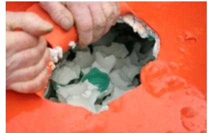
The interior of a damaged flotation system of the mooring M7. Photo: Joel Sudre
