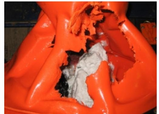
An imploded buoyancy element from a mooring, the glass sphere of which is transformed to a sand-like glass cake. Photo: Charlotte Lohse
