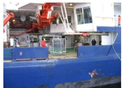
The CTD to measure vertical profiles of temperature and salinity as well as to take water samples is lowered from board. Photo: Charlotte Lohse
