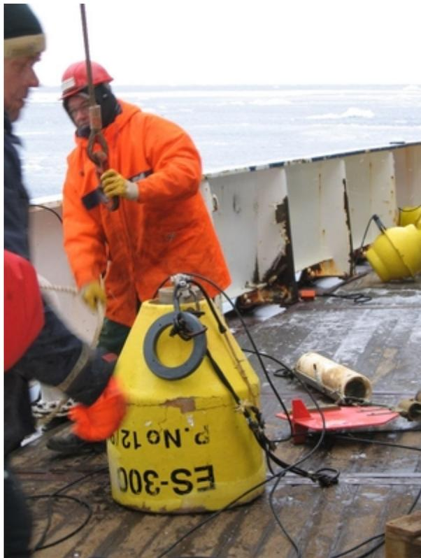
The upward looking sonar and a current meter from the mooring which was dragged away by an iceberg. (photos: Charlotte Lohse)
