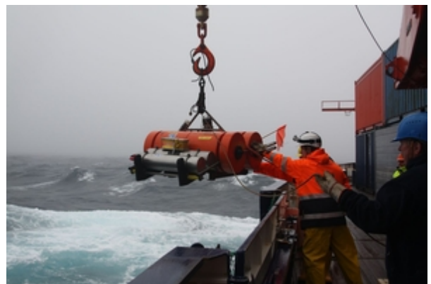
Fig. 1: Deployment of an ocean bottom seismometer at the stormy Southwest Indian Ridge. (Photo: F. Mehrtens, AWI).
