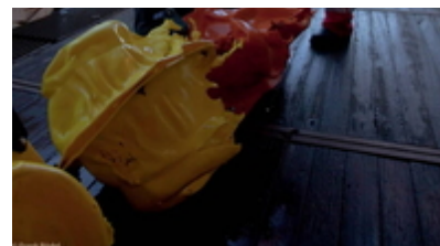
Fig. 2: The oceanographers are concerned by the imploded glass floats (Photo: Frank Rödel).
