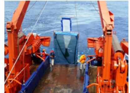
The Rectangular Midwater Trawl is deployed from the aft. (photo: K. Hammrich)
