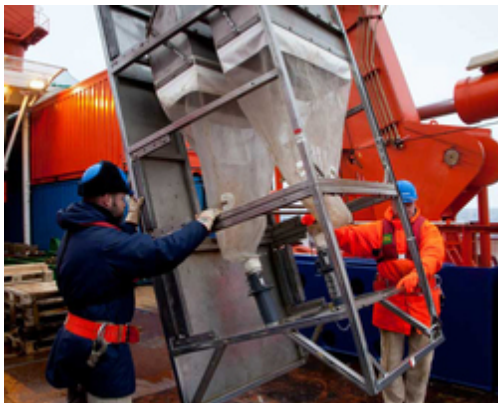
The Epibenthos Sledge is carried to the aft to be deployed. (photo: F. Rödel)
