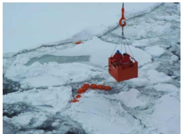
Recovery of a mooring in the ice by means of the mammy chair. (photo: E. Fahrbach)
