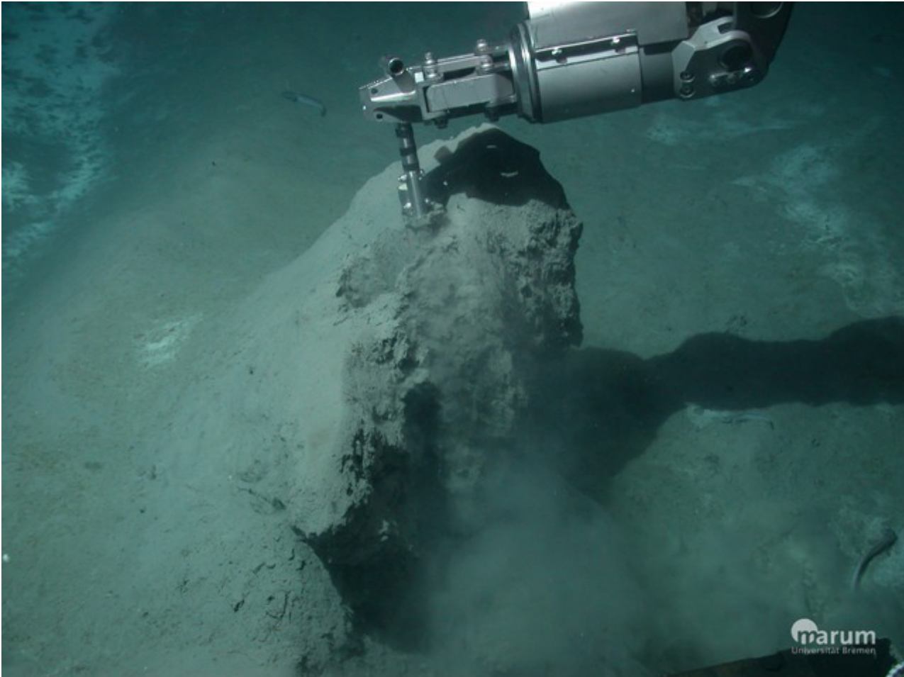
Sampling of a large hydrate and gas structure which has emanated from the seafloor.
