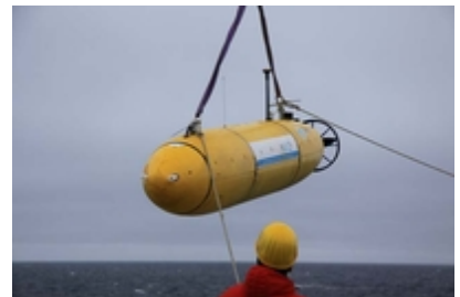
The deployment of the Autonomous Underwater Vehicle is supported by the ship crew keeping the ropes tight.
