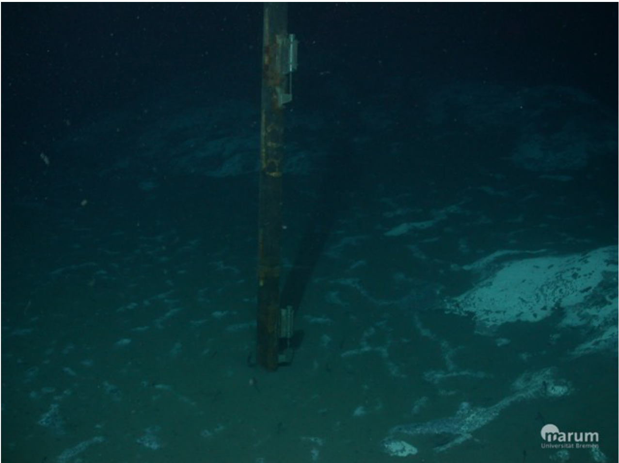
The IFREMER temperature lance after one year of deployment, shortly before its recovery by QUEST. It has penetrated gas hydrate and measures subsurface and surface temperatures.
