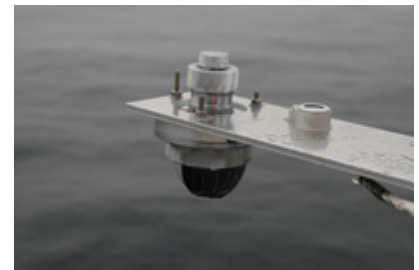
Pyranometer measures the reflected solar radiation from the sea surface. Photo: Niko Renkosik
