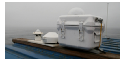
On the left hand side the pyranometer (solar radiation) and the pyrgeometer (longwave radiation), on the right hand side the full sky imager with a fish-eye objective. Photo: Niko Renkosik
