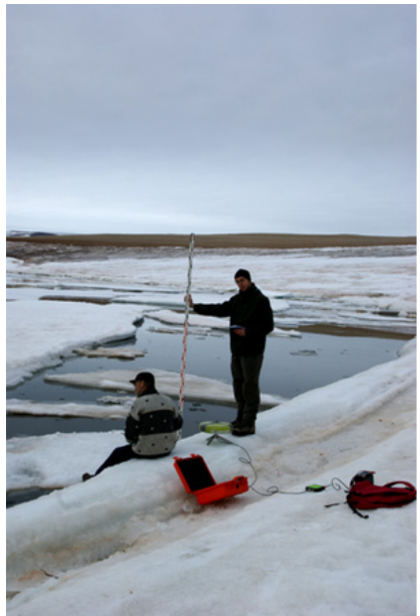
Holmland - Temporary installation of a tide gauge in a bay of Holmland. With tide gauge data and repeated measurements in the following years, it can be calculated, if the sea level rises or falls. Photo: Kristin Novotny
