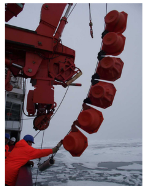
...and buoyancy flotations with acoustic transponder in the western Fram Strait. Photos: A. Beszczynska-Möller, AWI (OZE)
