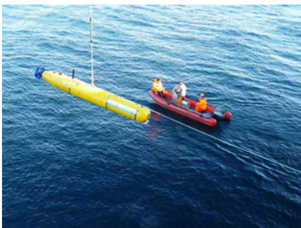
The Autonomous Underwater Vehicle (AUV) being recovered after a dive at 500 m water depth. Assistance by a team in the Zodiac is necessary to hook the vehicle to one of the ship's crane. (Photo: M. Klages)
