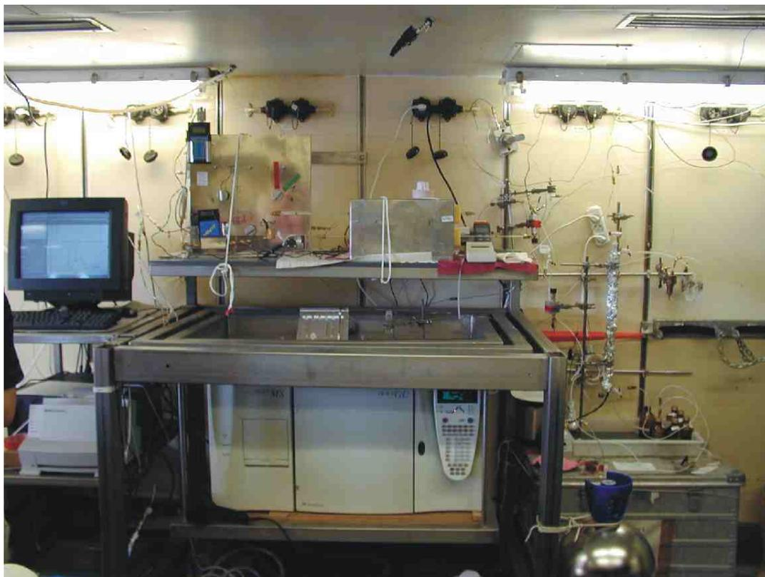
**Abbildung 2: Gas-chromatograph/Mass spectrometer system in the GeoLabor.**
