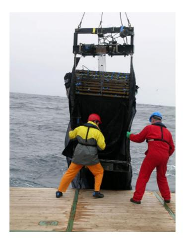
Figure 3: Deployment of the 1m<sup>2</sup>-MOCNESS with 9 netbags.
