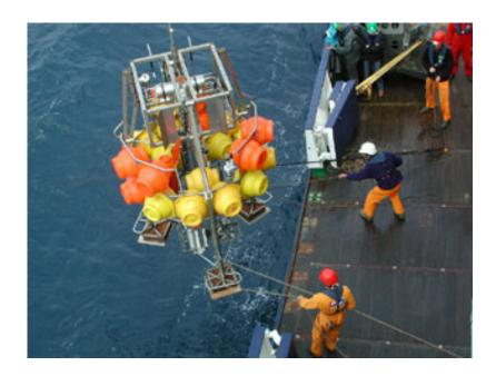
**Figure 4**: Deployment of a GEOMAR BC-Lander carrying an OceanLab bioluminescence observatory.
