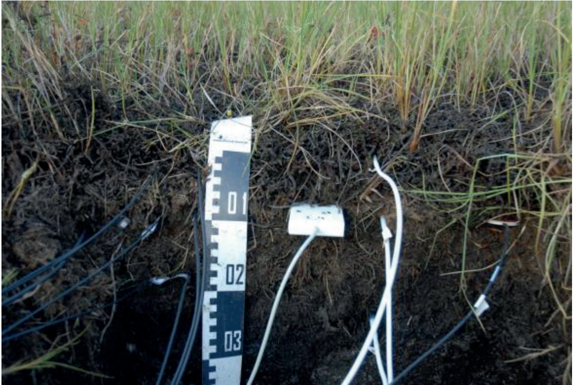
Figure 3-10 Instrumentation in upper soil of center profile. From left to right: oxygen probes, white “box” TDR probes (white boxes), PT100 temp probes (white cables), heat flux plate.
