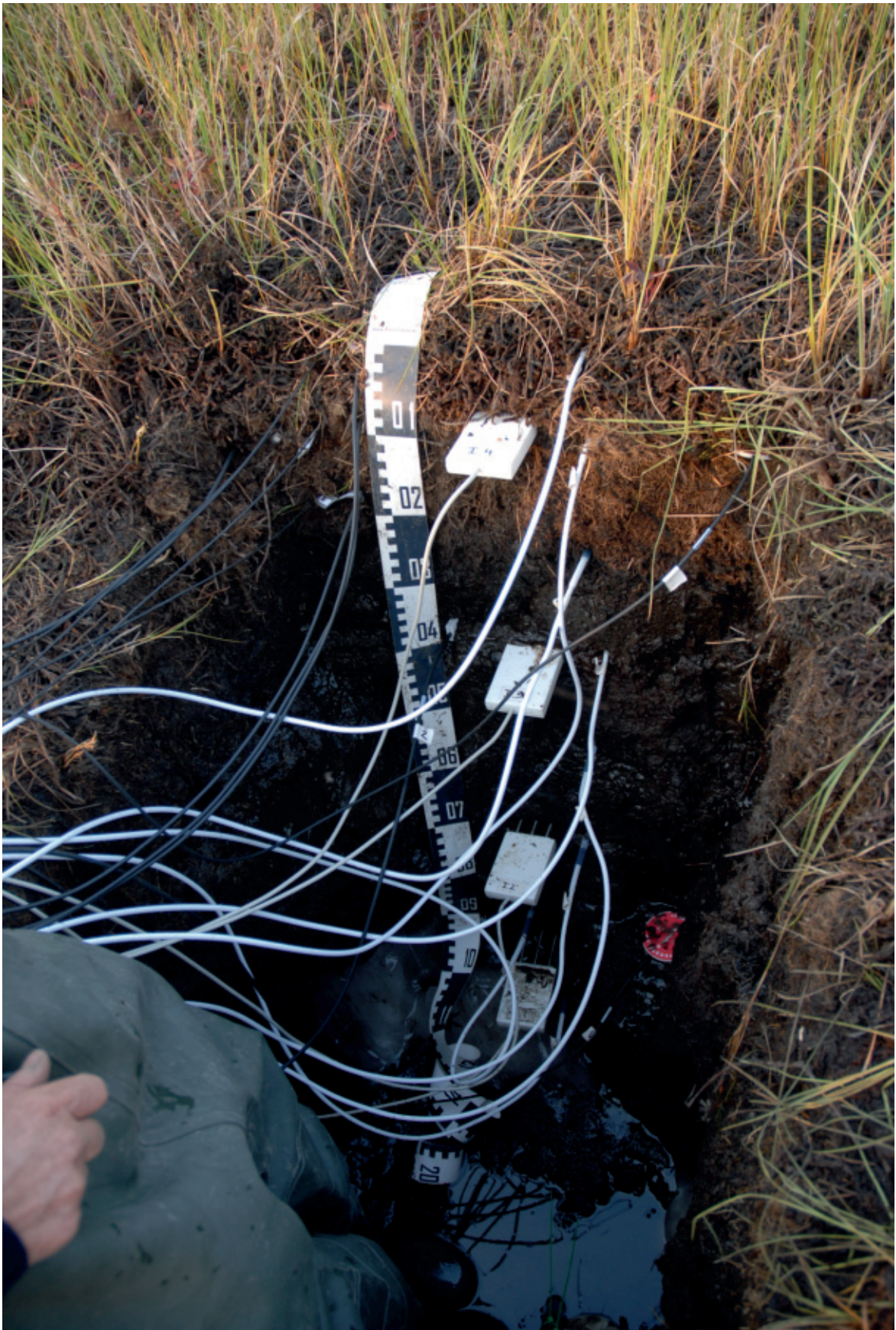
Figure 3-9 Fully installed center profile. Frozen ground was encountered at about 41 cm below ground surface corresponding to the second TDR sensor (from top down).
