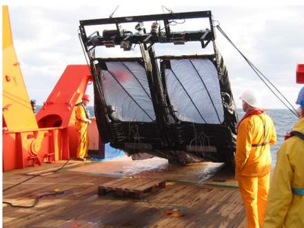
not allow for using towed gear, so we started with several CTD/rosette casts. On the following day, the weather and sea conditions improved considerably, and one 10 m<sup>2</sup>-MOCNESS haul (down to 1000 m) and two hauls with the 1m<sup>2</sup>-double-MOCNESS (down to 4170 m) could be performed.
